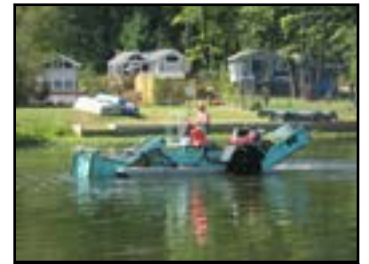
Figure 6. Woodhaven's aquatic plant harvester out on one of the lakes removing vegetation.
